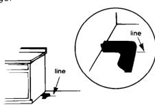
• Place one end of the anti-tip bracket on the floor against the cabinet side so that the inside edge of the bracket is aligned with the line drawn.
